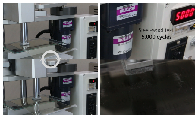
Figure 1. Procedure of steel-wool scratch test (left) and excellent scratch resistance of Flex9H ® (right).
